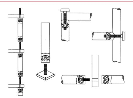
Inside Tube Diameter = 24,6-25,6Outer tube diameter =  $1 \ 1/8$ " Thread = M6
